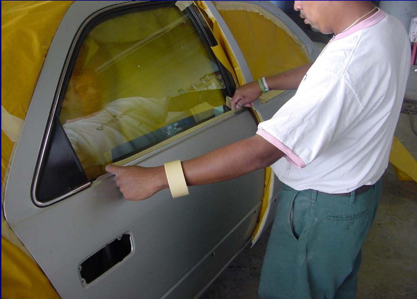
The technician is masking off the rear door glass.
