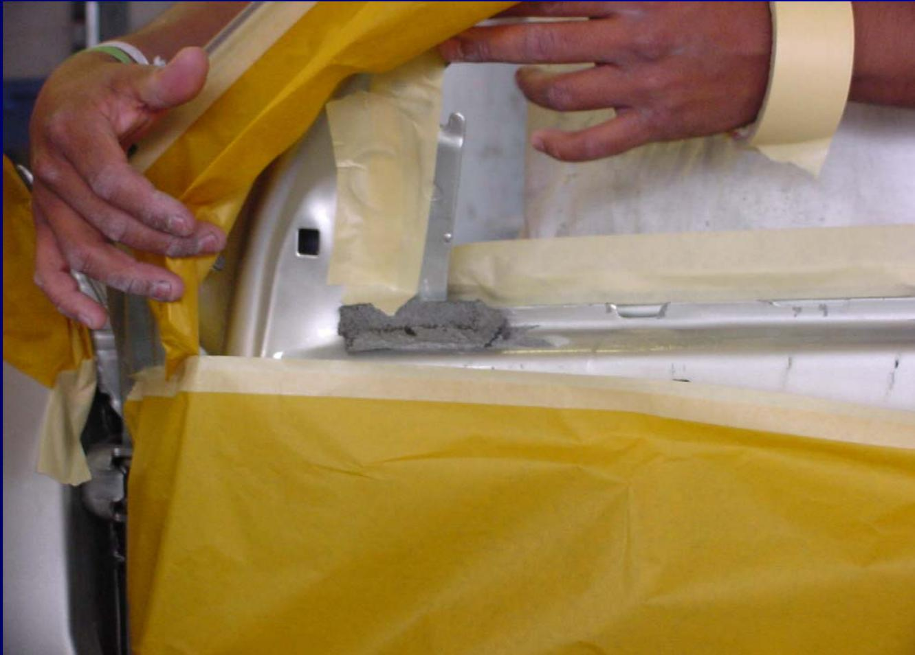
Technician is masking off the front door jamb.
