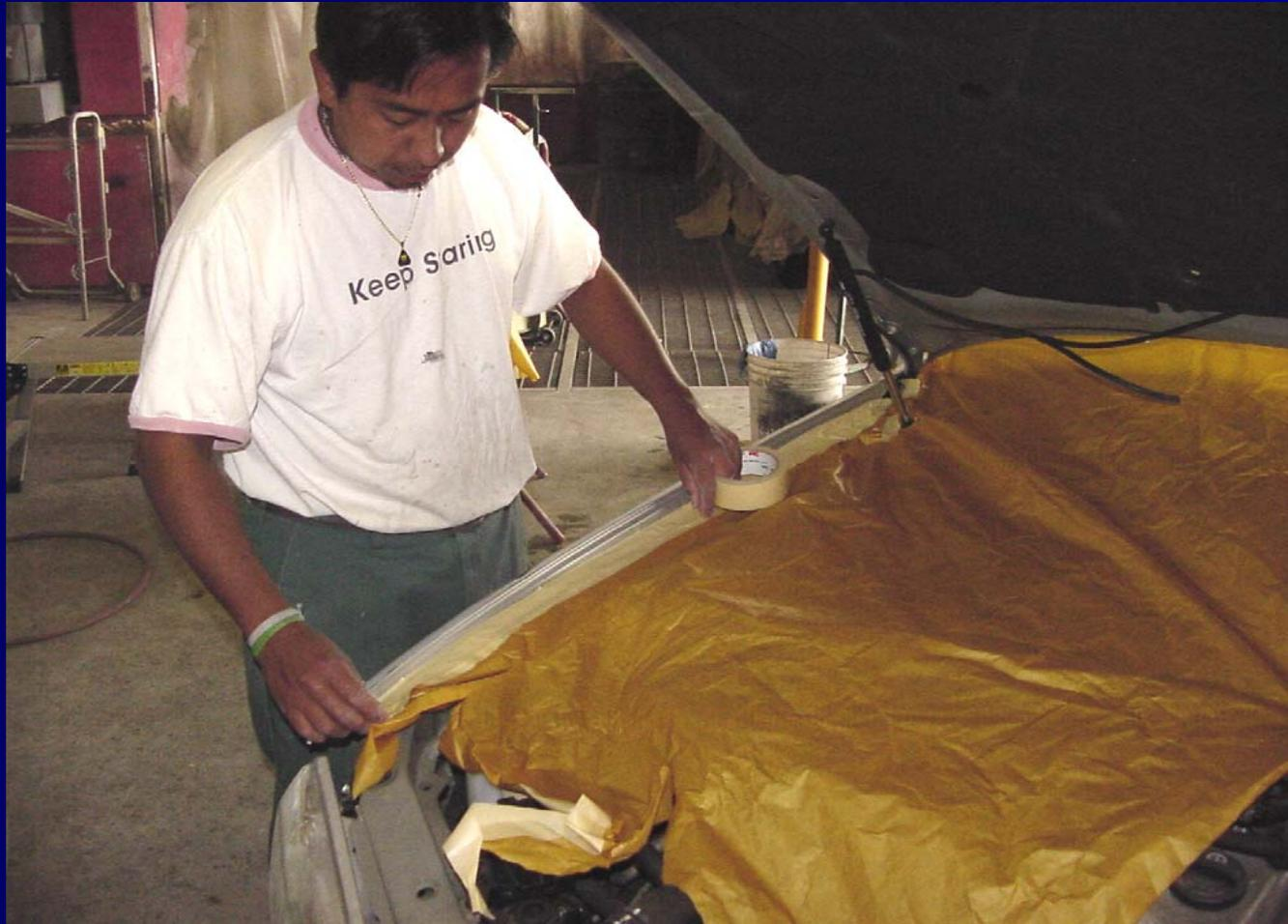
Technician is masking off the engine.
