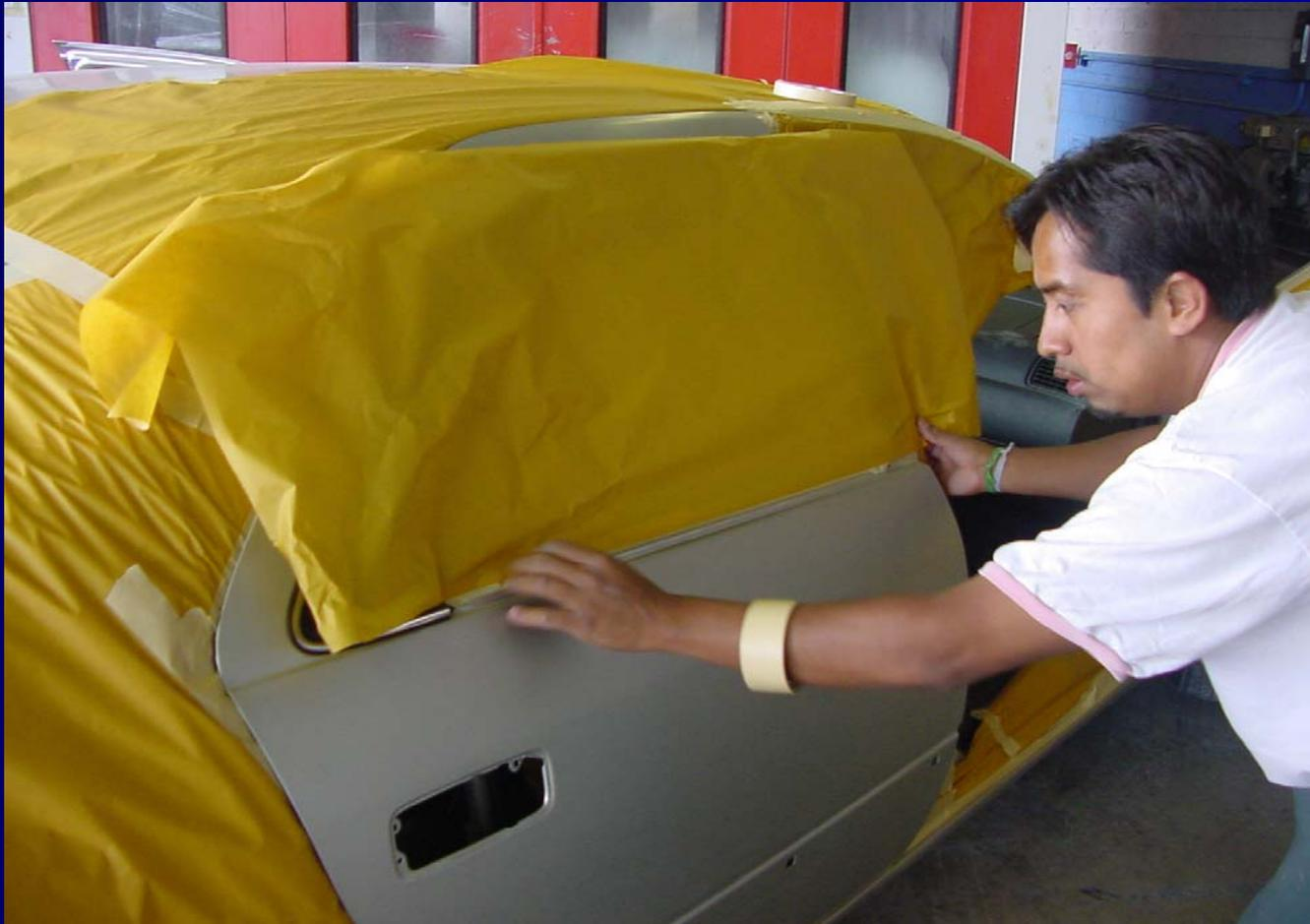
The technician is applying fine line tape to the door frame molding.
