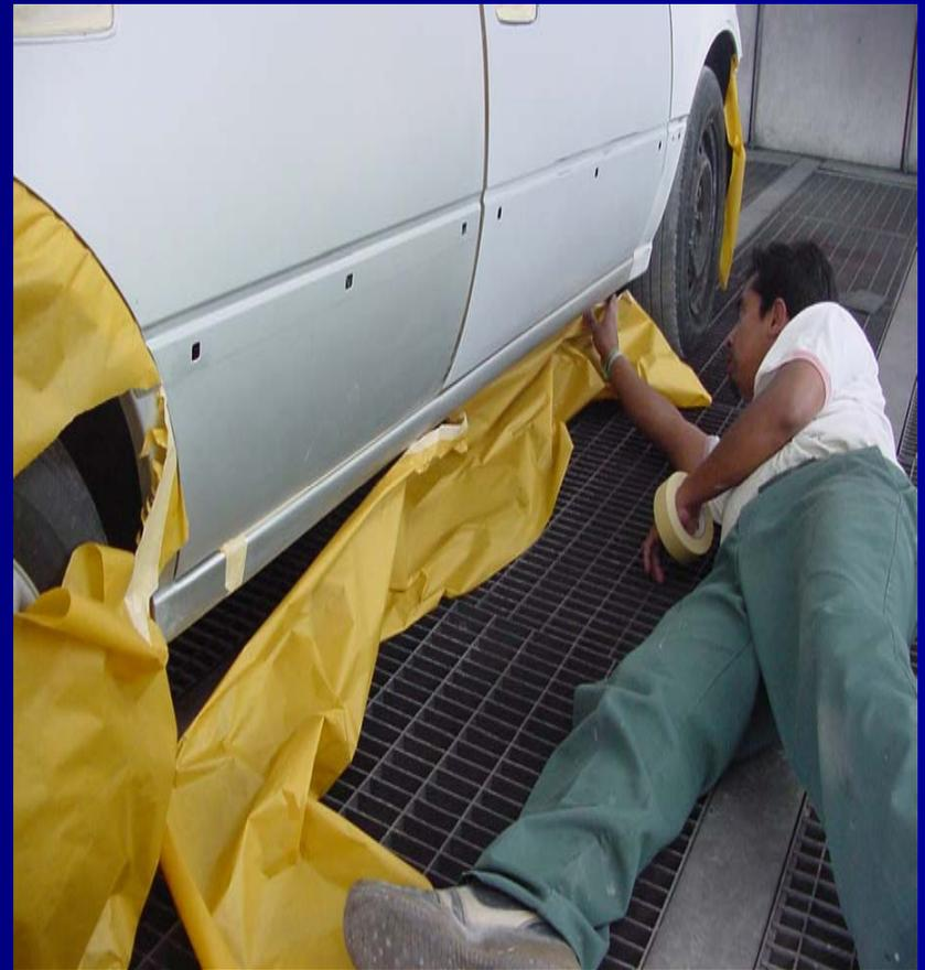
The passenger's side fender and tire are masked off.
