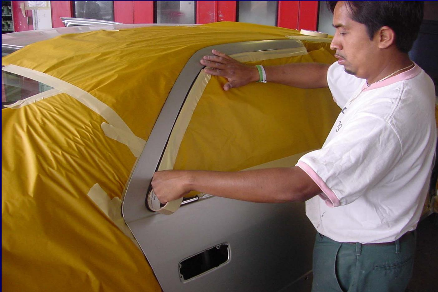
Technician is applying tape to the door handle opening.
