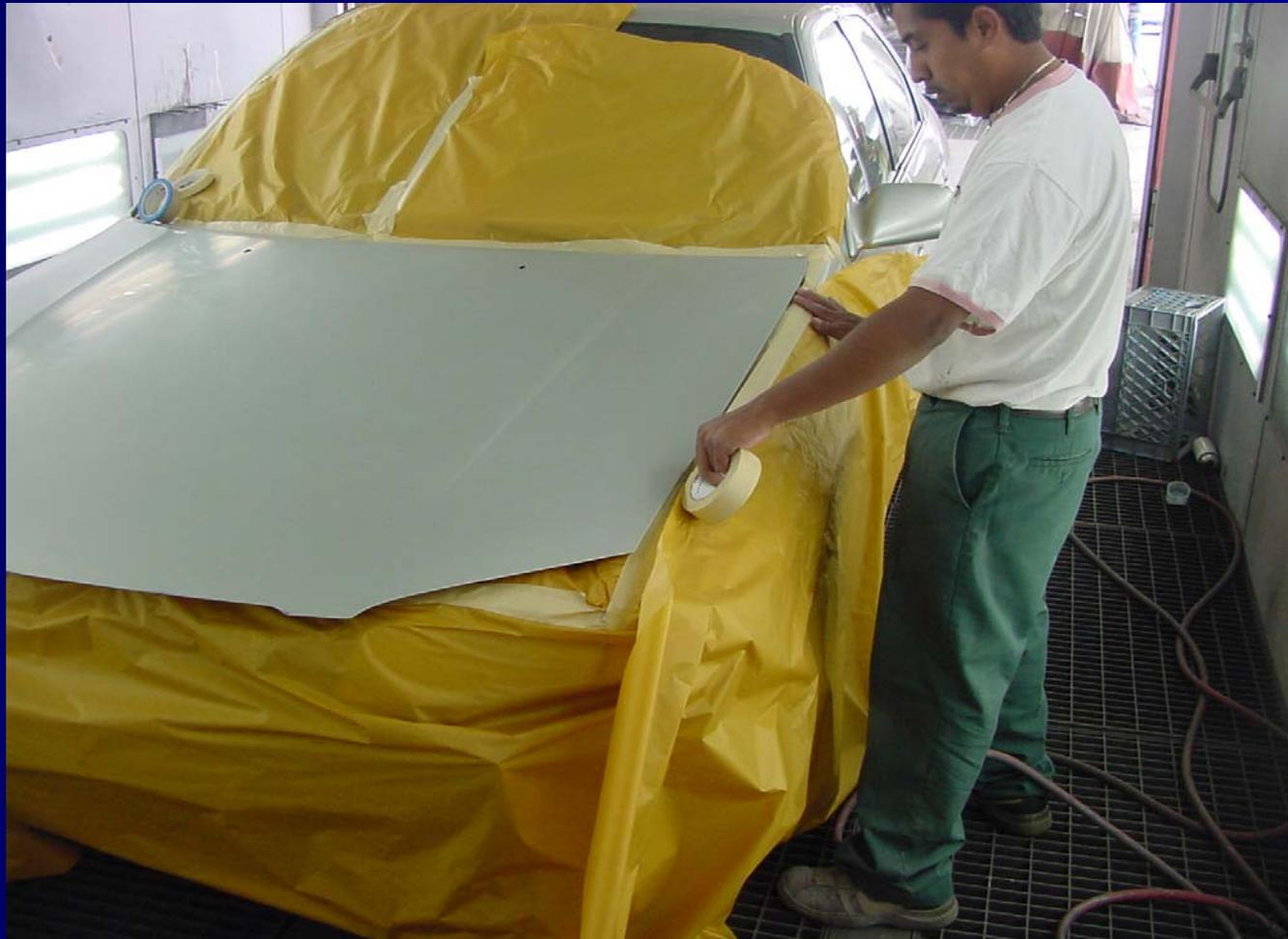
Technician is securing the plastic cover to the vehicle.
