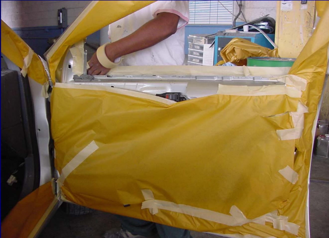
The technician is applying tape to the mirror opening hole.
