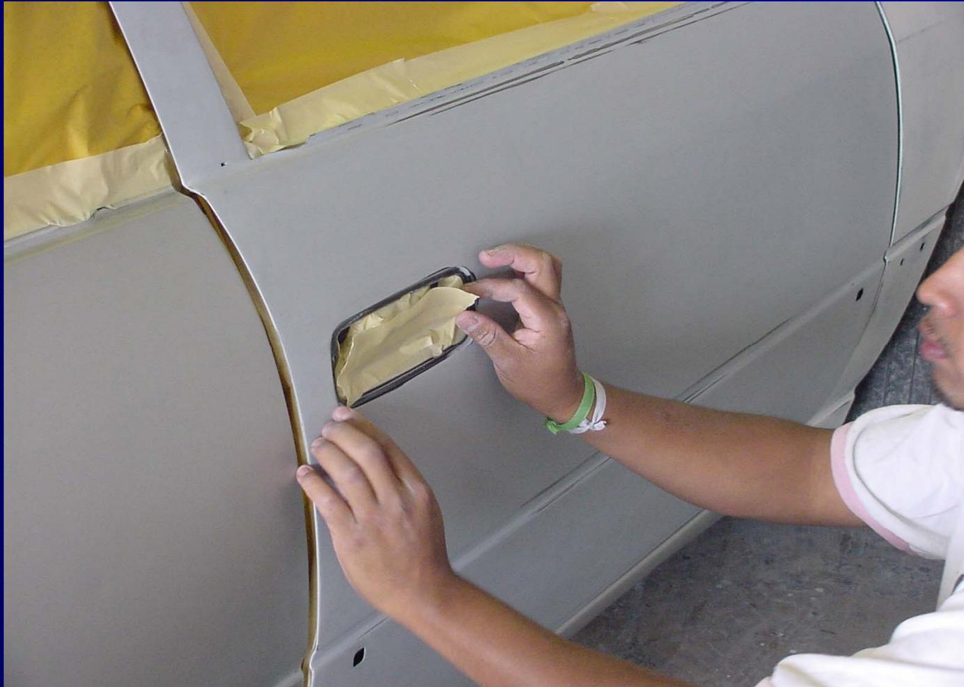
The technician is applying tape to inner belt molding edge to secure masking paper.
