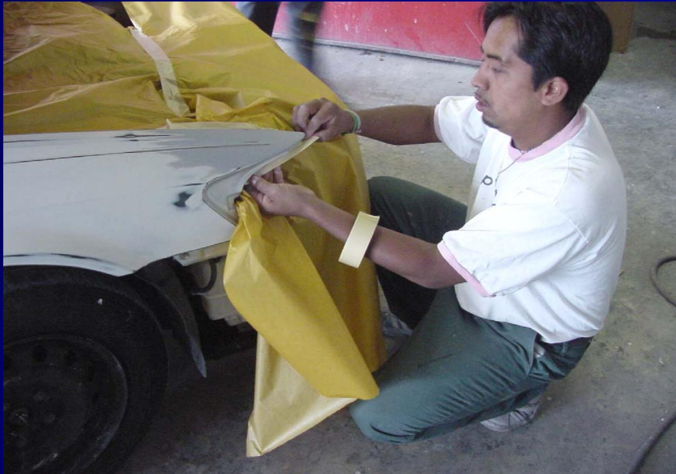
The technician has tapped off the inner door frame.
