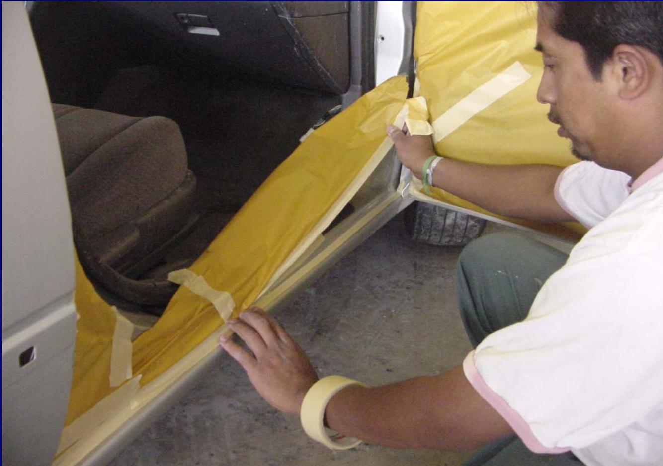
The technician is applying tape to the front door window opening lip in order to secure the paper to the opening.
