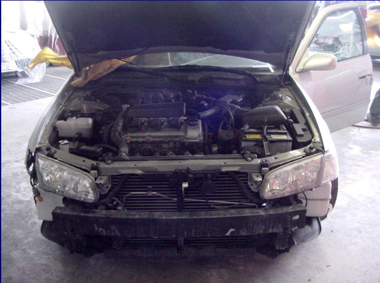
The technician is beginning the masking off of the engine compartment.
