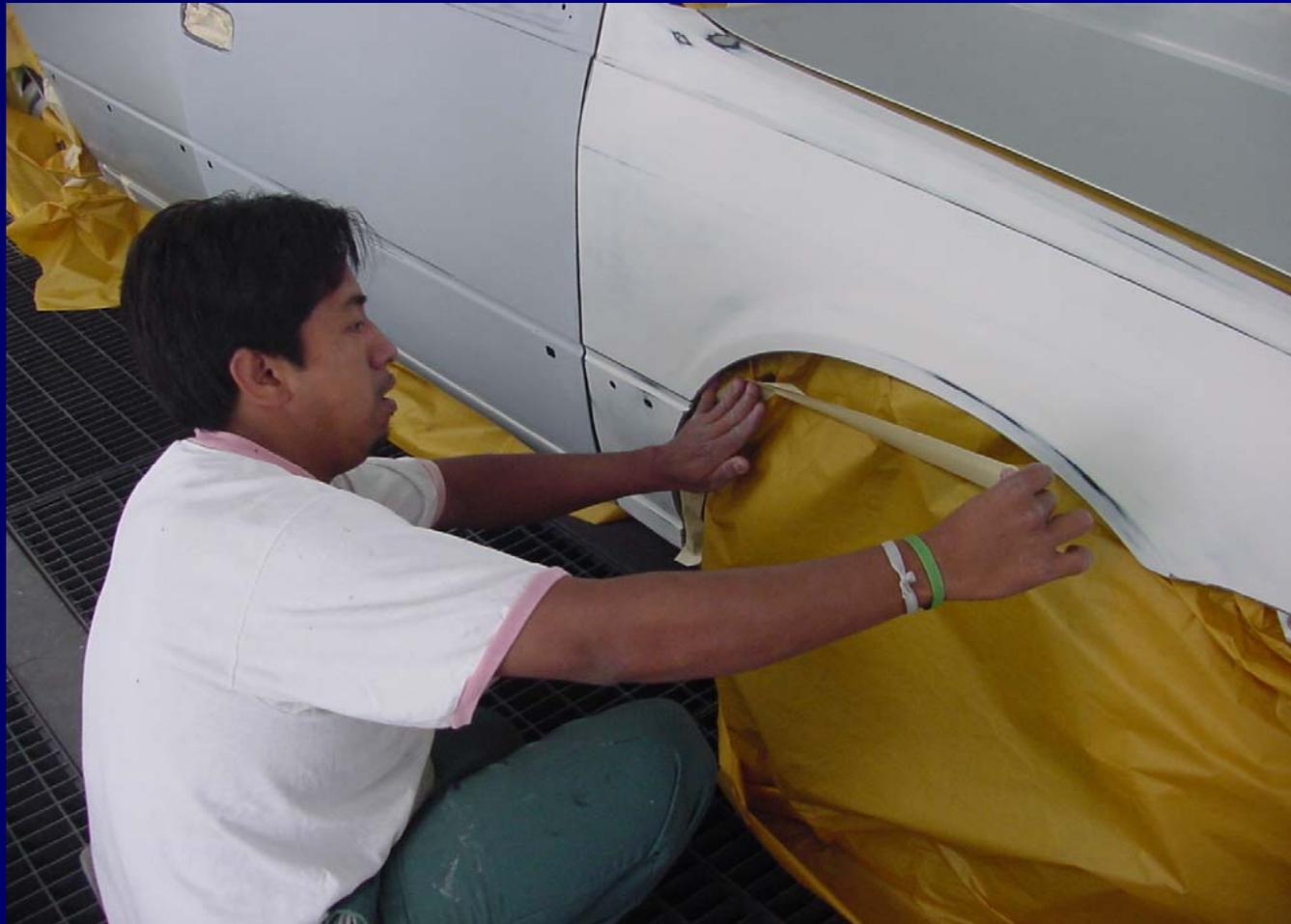
The passenger's side front fender and front core support are masked off.
