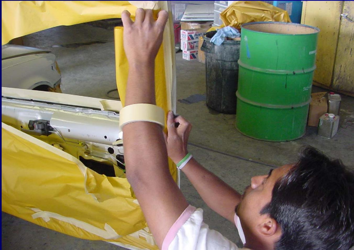
Technician is applying masking paper to the inner rocker panel.
