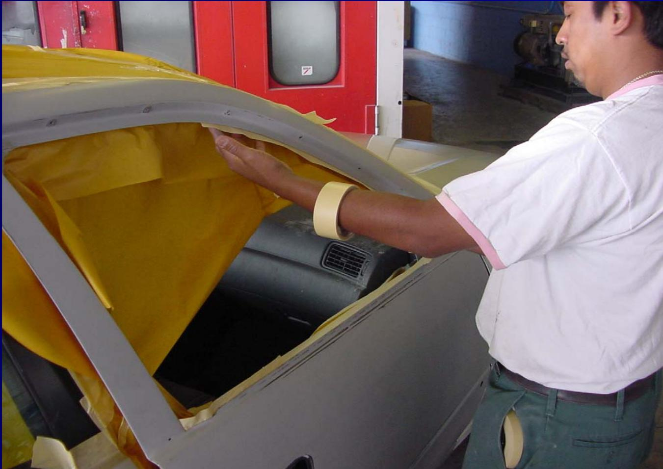
The technician is applying masking paper to the window opening.
