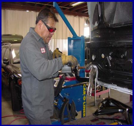
The second option is to use a MIG welder with 8 MM plug welds. Since this inverter resistance spot weld technology is new, the rest of the presentation will concentrate on the plug weld option which is more widely used by the collision repair industry.
