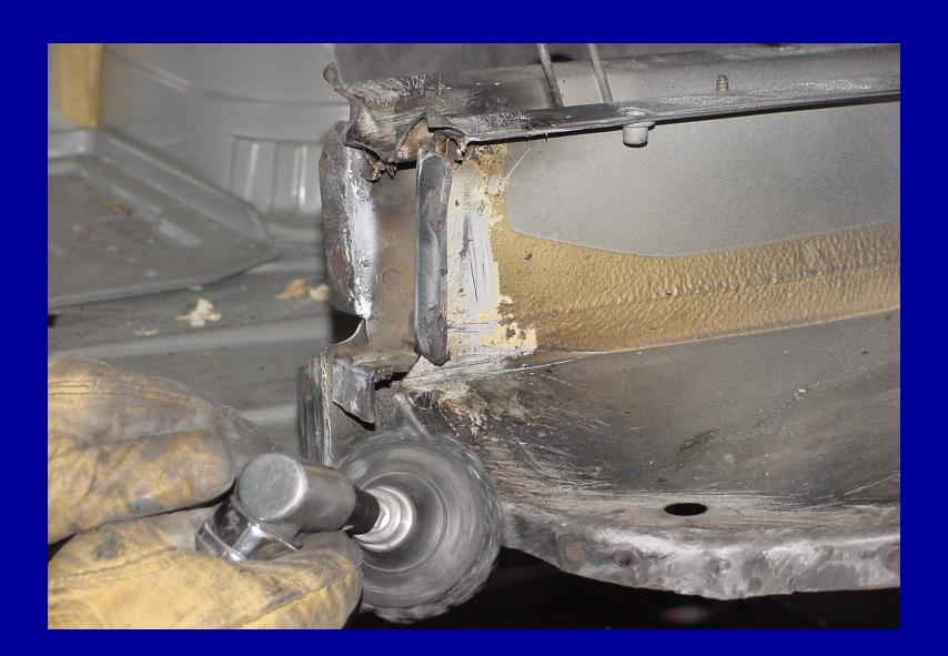
At this point there are 2 options available for the technician to install the inner Boron Steel rear body panel: First he/she can use a resistance spot welded that will work on Born Steel or
