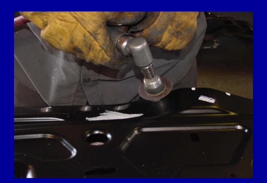
Plug weld the frame rail to the rear body panel (it was easier for the tech to drill holes in the frame rail ends instead of rear body panel).
