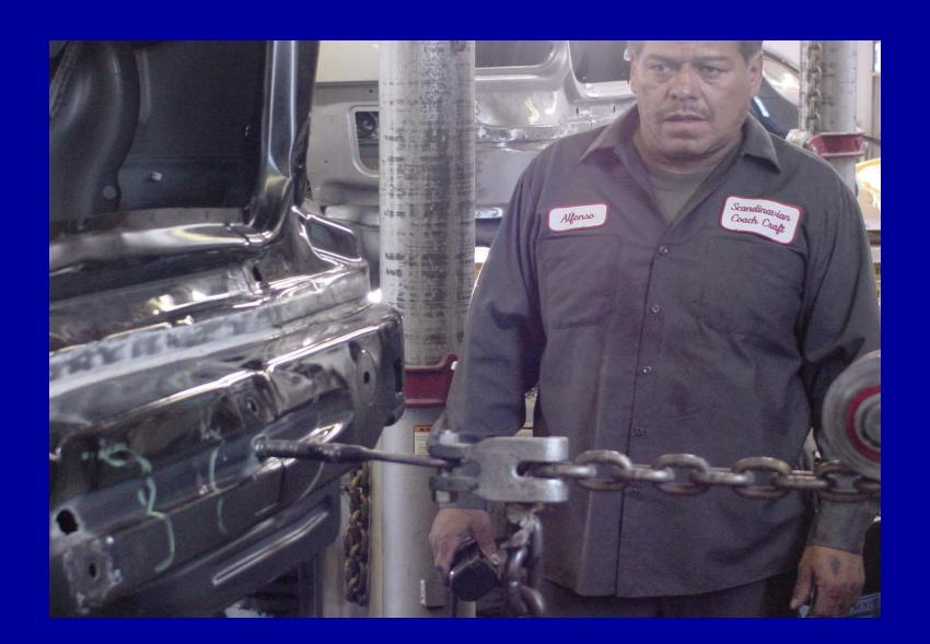
Note how bumper reinforcement is over pulled but returns to its original damaged state after the pressure is relieved.
