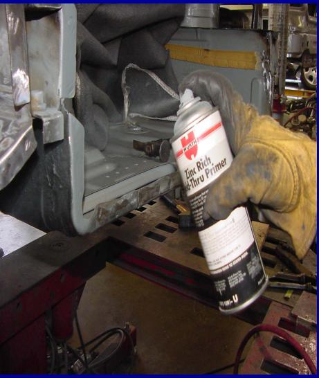
Clean inner panel that is to be plug welded to remove the weld thru primer from the weld site as recommended by I-CAR.
