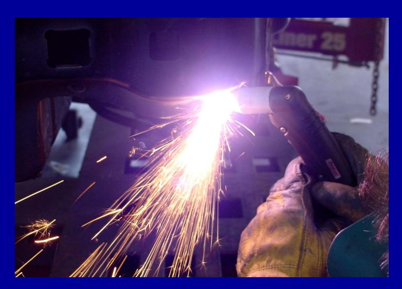
Remove portion of outer bumper reinforcement to expose sport welds the attach the inner panel to the frame rail.
