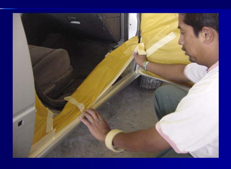
The technician is applying tape to the front door window opening lip in order to secure the paper to the opening.
