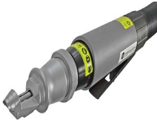
The **MEC600** pneumatic milling cutter tool has been designed to open welding seams for easy removal of the outer panels. The adjustable guide of the cutter allows the **MEC600** to be easily adjusted to different angular positions of the metal sheets and no damages by preventing the cutter from slipping off the edge.
